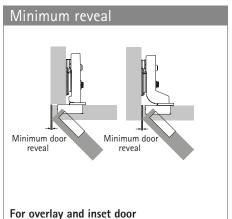
The minimum reveal (also known as the door clearance or minimum clearance) is the space required at the side for opening the door. The size of the minimum reveal depends on the cup distance C, the door thickness and the type of hinge selected. Radii on the door edges reduce the door clearance. The minimum reveal is shown in the table for the respective hinge types.
